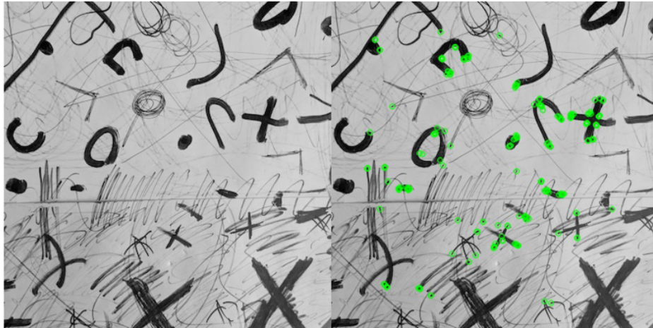
Fig. 20 An image taken on the drone's camera, shown with and without plotting the coordinates of 200 features detected by ORB
