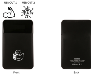
Fig. 66 Duckiebattery outputs behave differently.
