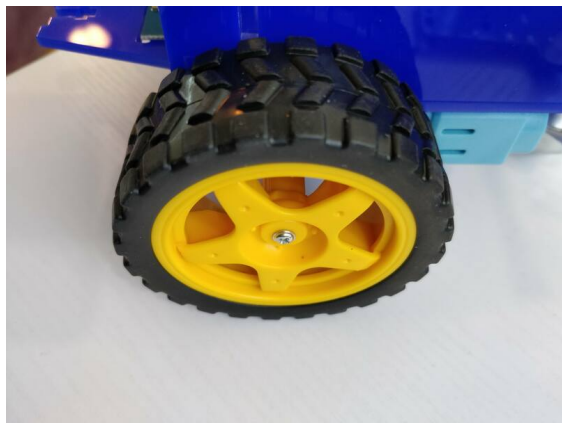
Fig. 36 Screws will keep the wheels in place. Do not tighten too hard!
