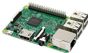
Fig. 8 The Raspberry Pi 3 Model B is a 1.2GHz, 64-bit quad-core ARMv8 CPU, 1GB RAM little computer.
