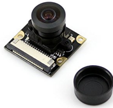
Fig. 13 The Raspberry Pi camera with fisheye lens.
