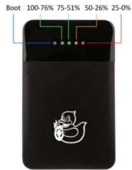
Fig. 63 LEDs indicate the state of charge of the Duckiebattery.
