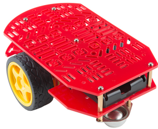
Fig. 7 The "Magician" chassis was very popular. It is used in DB17 through DB19 Duckiebot models.
