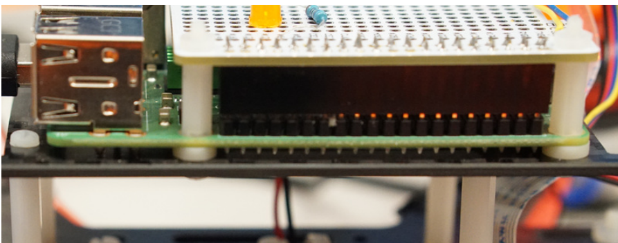
Fig. 100 Raspberry Pi mounted on the upper frame (with Raspberry Pi Hat)
