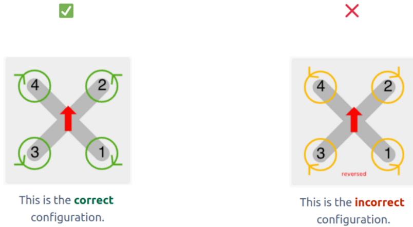
Fig. 89 Motors correct spin direction
