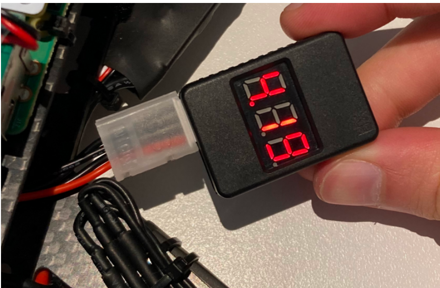
Fig. 111 Battery connected to the Battery Monitor
