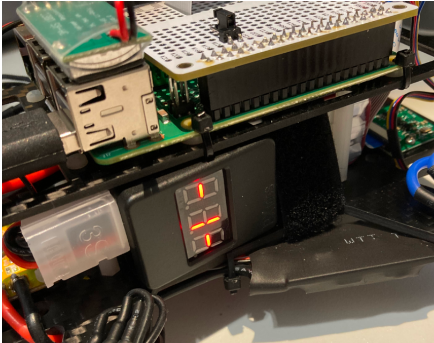
Fig. 112 A possible location to attach the Battery Monitor
