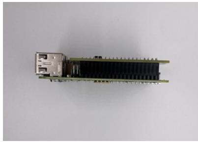
Fig. 47 Raspberry Pi Hat inserted into Raspberry Pi pins
